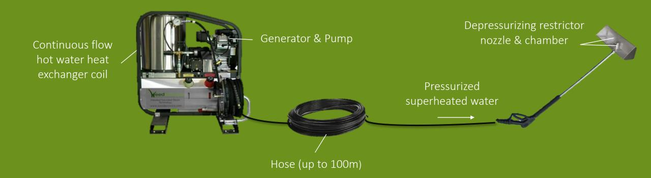
Produces highly saturated Satusteam™ at 98-110°C/210-225°F just 1-2" from the weed for highly impactful **Thermal Shock**
