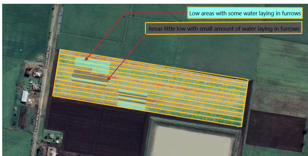
Figure 7: Drainage findings from a drone flight in January 2019
