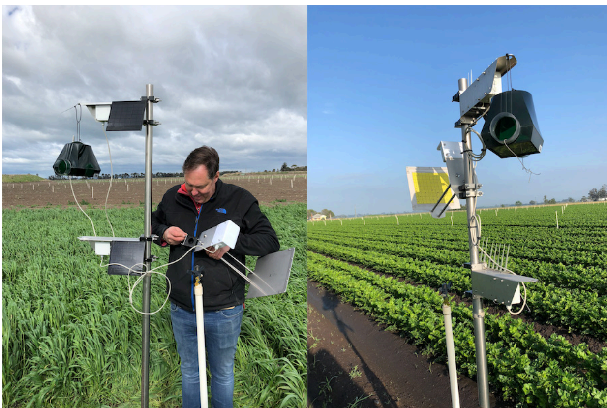
Figure 9: The remote monitoring insect trap being installed in August (left) and in full-swing during December 2018 (right)
