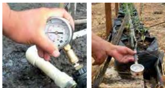
Monitoring pressure at the beginning of a lateral and at the end of a lateral.
