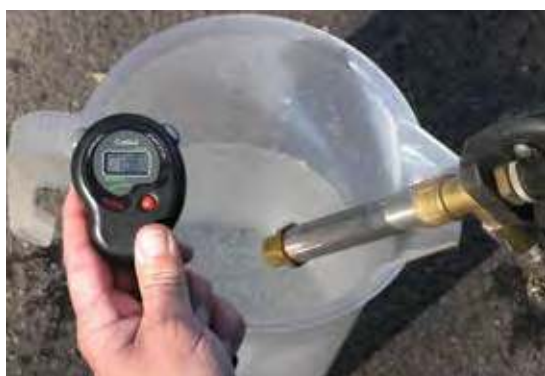
Step 1: Using water, measure how many litres are emitted into a measuring jug from the sprayer in one minute. This is the nozzle output.
