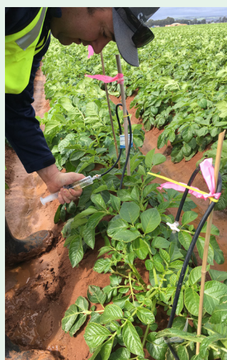
Figure 3: Extracting soil water from installed solusamplers in fresh market potatoes of South Australia.
