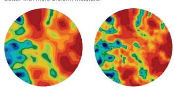
Figure 2: Electromagnetic Induction surveys at 100cm (L) and 50cm (R) depths, showing the spatial variation in soils and likely areas of salinity.
