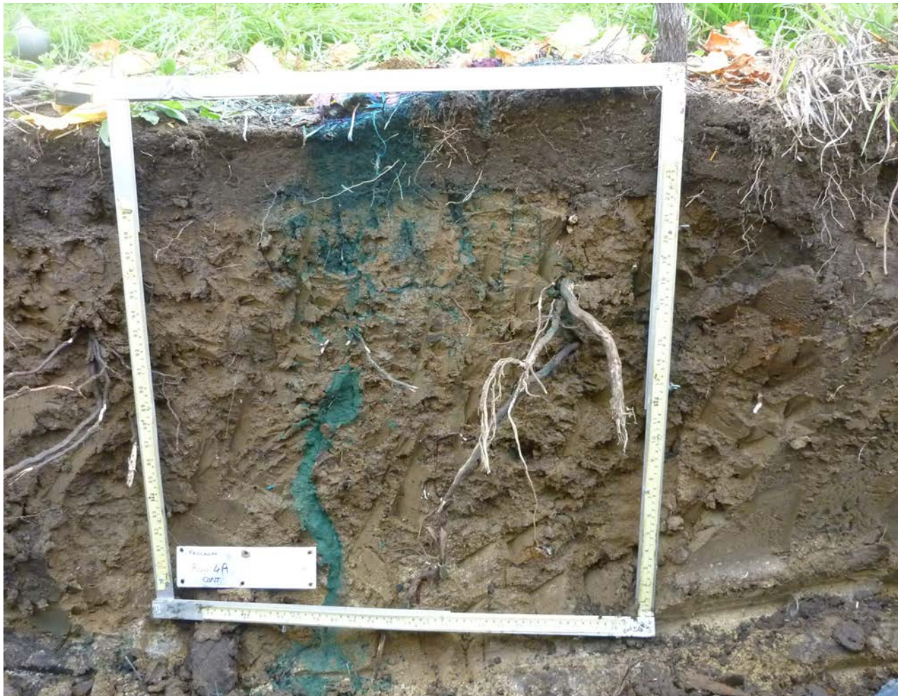
Figure 1-3. Soil water profile illustrating variability in distribution and infiltration (Photo courtesy: Marcus Hardie, University of Tasmania)
