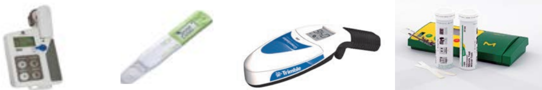
Figure 8-5. Some examples of field-based instruments (left to right): SPAD 502 - chlorophyll density (Minolta), Cardy Nitrate meter – sap nitrate (Horiba), Greenseeker – NDVI (Trimble), Merck Reflectoquant® spectrophotometer (Merck KGaA)
