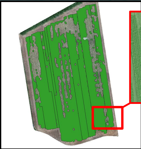
Spot spray Nitrogen map: Green colour corresponds to the Nitrogen spray being applied.
