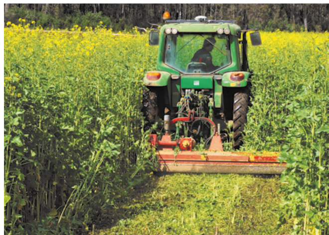
Mulching of a high biomass cover crop using a flail mower to produce fine residues.
