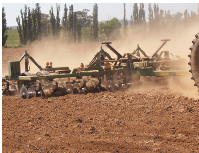
Supercolter lightly working in cover crop residues after discing.
