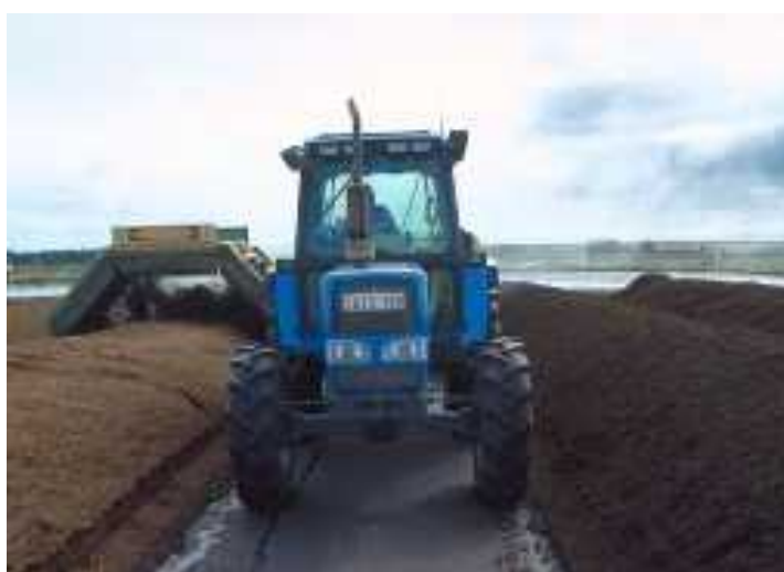
Figure 6. Tractor-drawn windrow turner. (Custom composts, Mandurah)
