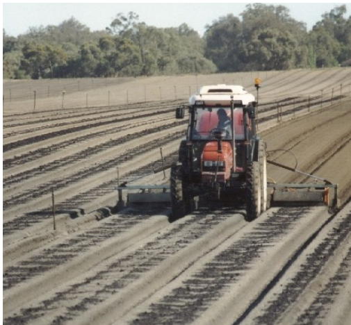
A bed rotary cultivator being used to lightly incorporate compost.
