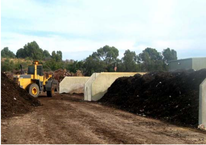
Figure 8. Static pile composting involves aeration with forced air. ( Biowise composting facility, Medina ).
