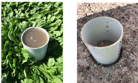
Figure 3 (left): Infiltration tests on 13 January 2021. Figure 4 (right): Infiltration tests on 22 January 2021. The soil surface shows signs of challenging conditions, especially soil structure.
