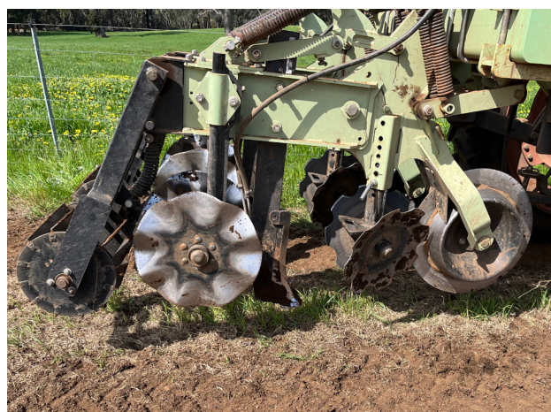
Figure 4. Strip till machine. Implements from R to L – straight depth coulters (cuts residue and maintains even depth), row cleaner (removes residue from strip), ripper shank (loosens soil), wavy coulters (controls tillage depth and width of strip), rolling basket (breaks clods and smooths surface)
