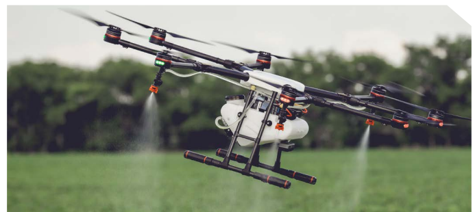
Figure 1. Use of GPS guided drones for precision spot spraying are on the increase. IMAGE: Adobe stock
