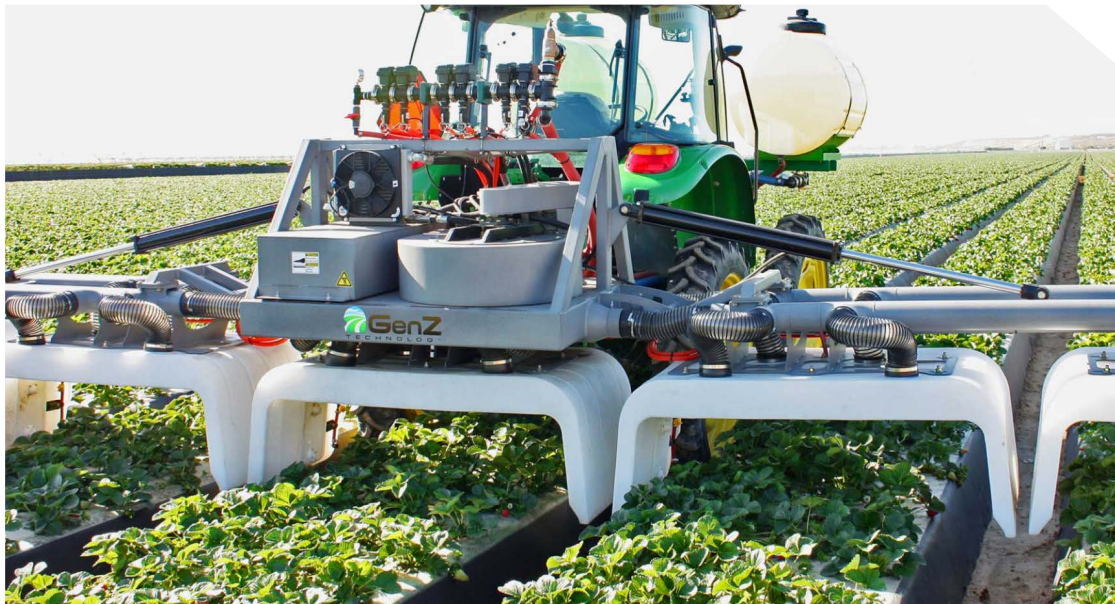
Figure 3. GenZ Smart Sprayer with hood that recaptures and recirculates excess spray reducing the risk of chemical drift. PHOTO: GenZ Technology.
