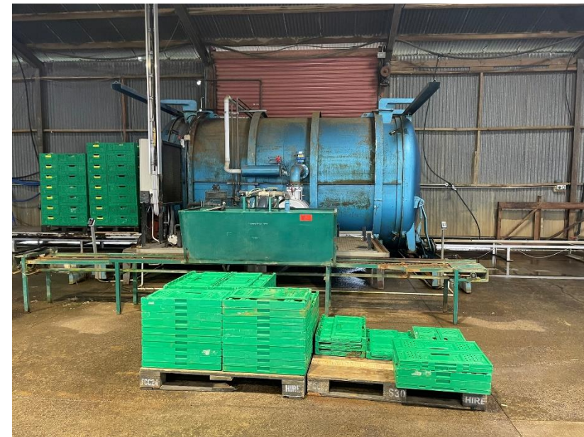
Vacuum cooling system
