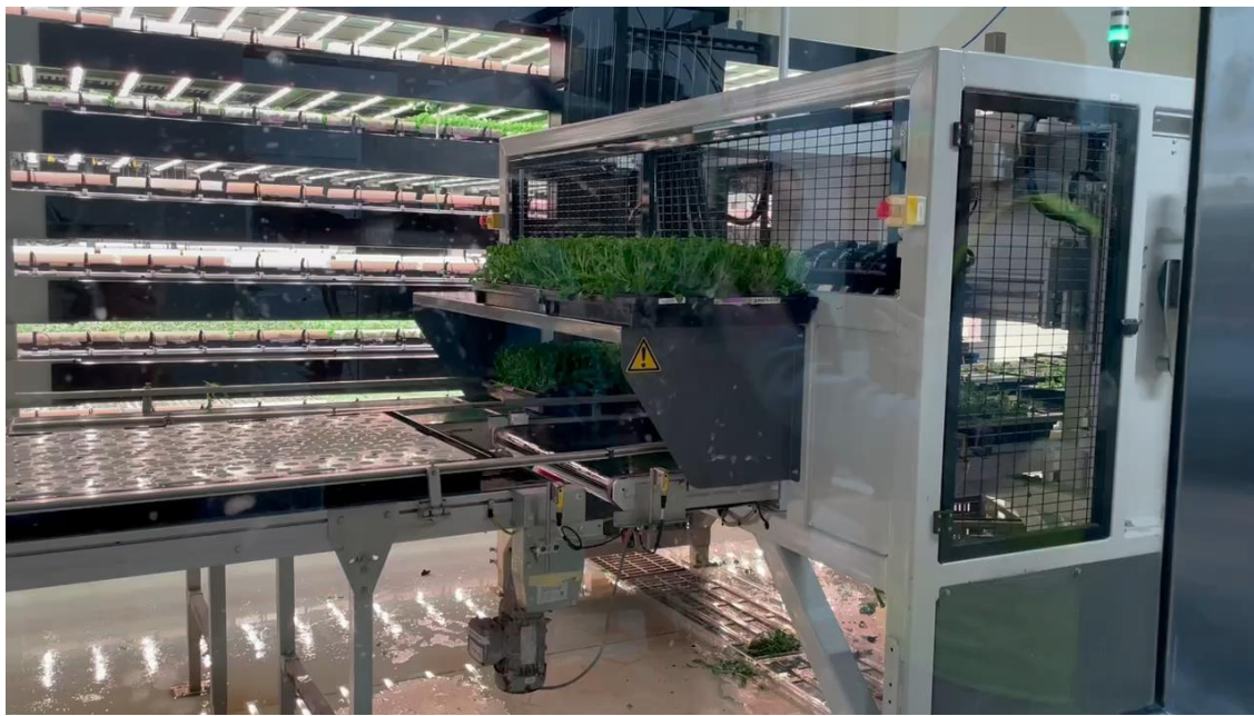
Seedlings are being transplanted from soil into trays for growth in a hydroponic system
